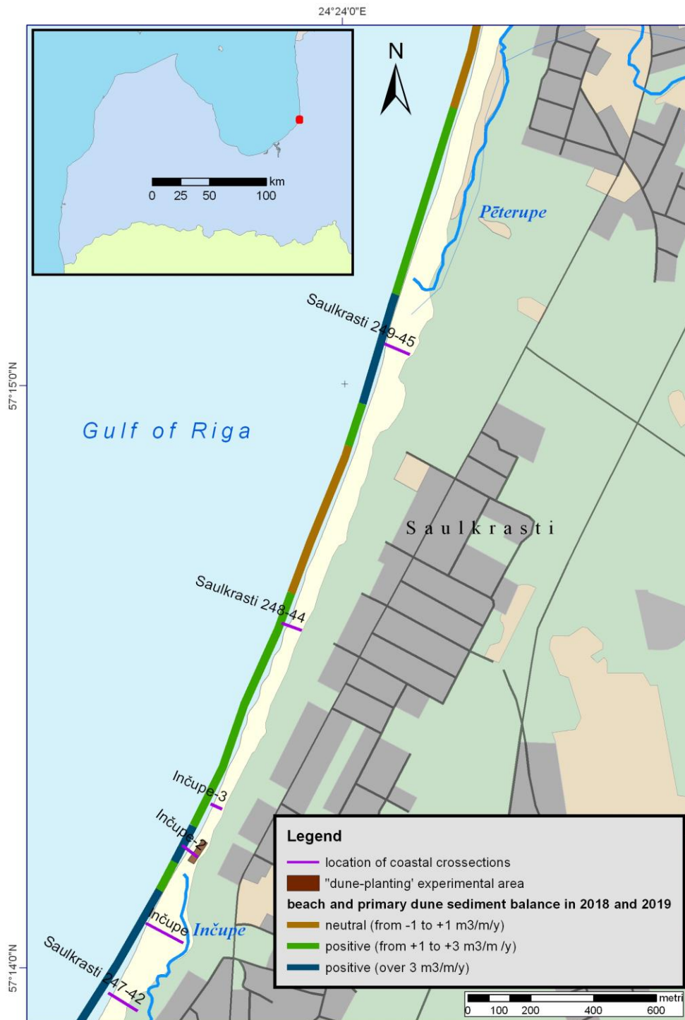
Figure 6. Beach and primary dune sediment balance in Saulkrasti Project implementation area coastal section during 2018 and 2019; location of cross-shore measurement profiles and “dune-planting” experiment site.
