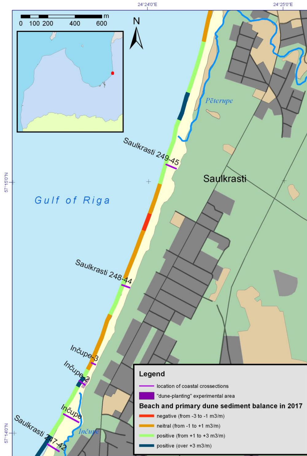
Figure 8. Beach and primary dune sediment balance in Saulkrasti Project implementation area coastal section during 2017; location of cross-shore measurement profiles and “dune-planting” experiment site.
